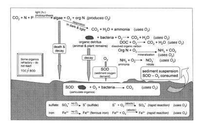
Conceptual Model of DO Depletion Reactions
